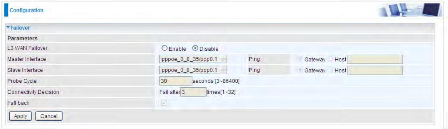
The screenshot shows the 'Configuration' page for 'Failover'. Under 'Parameters', 'L3 WAN Failover' is set to 'Disable'. 'Master Interface' and 'Slave Interface' are both set to 'pppoe\_0\_8\_35/ppp0.1'. For both interfaces, 'Ping' is selected, and 'Gateway' and 'Host' are empty. 'Probe Cycle' is set to '30 seconds [3~86400]'. 'Connectivity Decision' is set to 'Fail after 3 times [1~32]'. 'Fall back' is checked. 'Apply' and 'Cancel' buttons are at the bottom.
