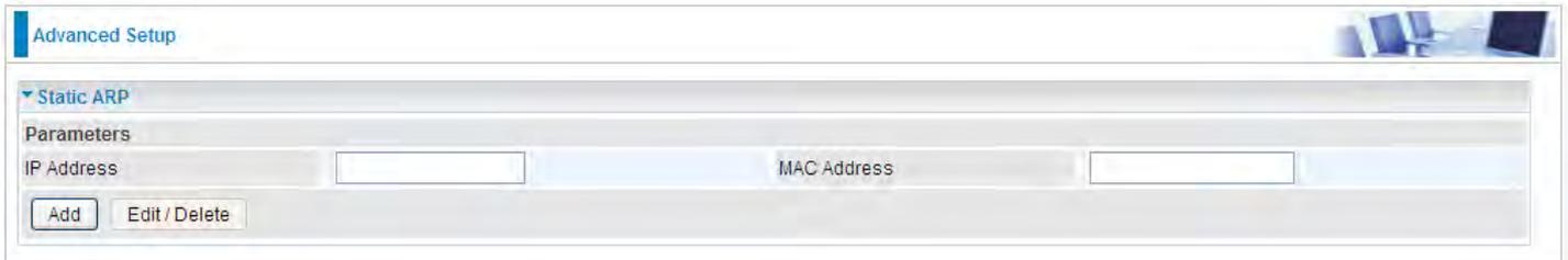
The screenshot shows a web-based configuration interface for Static ARP. At the top, there is a tab labeled "Advanced Setup". Below it, a section titled "Static ARP" is expanded. Underneath, a "Parameters" section contains two input fields: "IP Address" and "MAC Address". Below these fields are two buttons: "Add" and "Edit / Delete".
