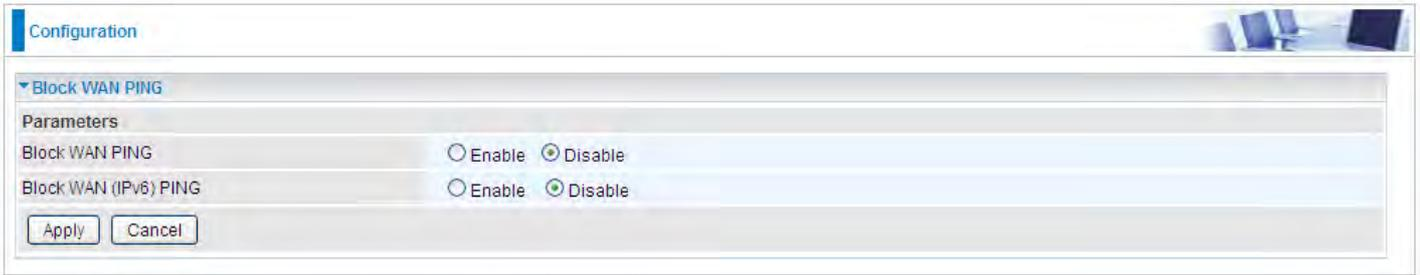
The screenshot shows a configuration window titled "Configuration" with a sub-section "Block WAN PING". Under "Parameters", there are two settings: "Block WAN PING" and "Block WAN (IPv6) PING". Both settings have radio buttons for "Enable" and "Disable". In both cases, the "Disable" option is selected. At the bottom of the configuration area, there are "Apply" and "Cancel" buttons.
