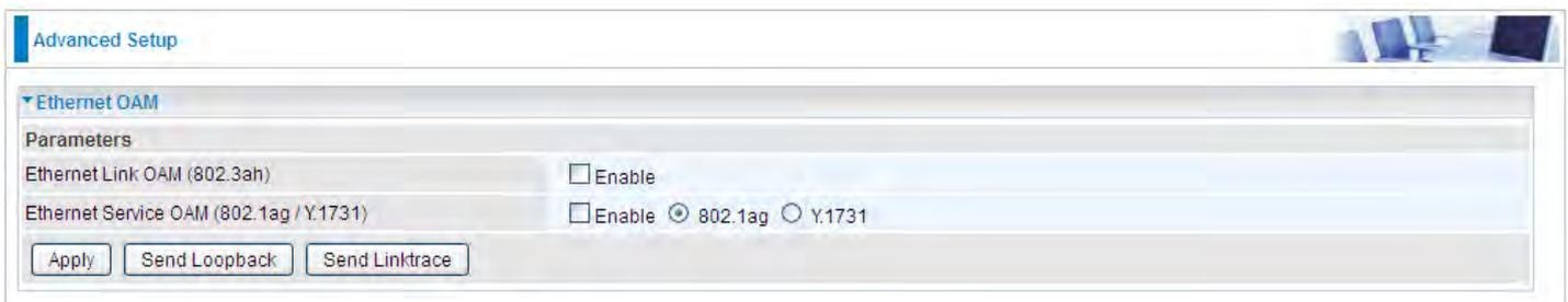
**Ethernet Link OAM(802.3ah):** Enable to activate Ethernet in the First Mile (EFM) Link OAM to do link fault management.
