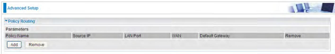
The screenshot shows the 'Advanced Setup' window with the 'Policy Routing' section expanded. Below the section title is a 'Parameters' table with the following columns: Policy Name, Source IP, LAN Port, WAN, Default Gateway, and Remove. Below the table are two buttons: 'Add' and 'Remove'.
