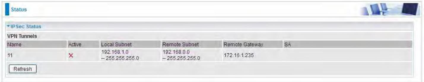
The screenshot shows a web interface titled "Status" with a sub-section for "IPSec Status". Underneath, there is a table labeled "VPN Tunnels". The table has six columns: Name, Active, Local Subnet, Remote Subnet, Remote Gateway, and SA. There is one row with the name "11". The "Active" column contains a red "X" icon, indicating the tunnel is inactive. Below the table is a "Refresh" button.
