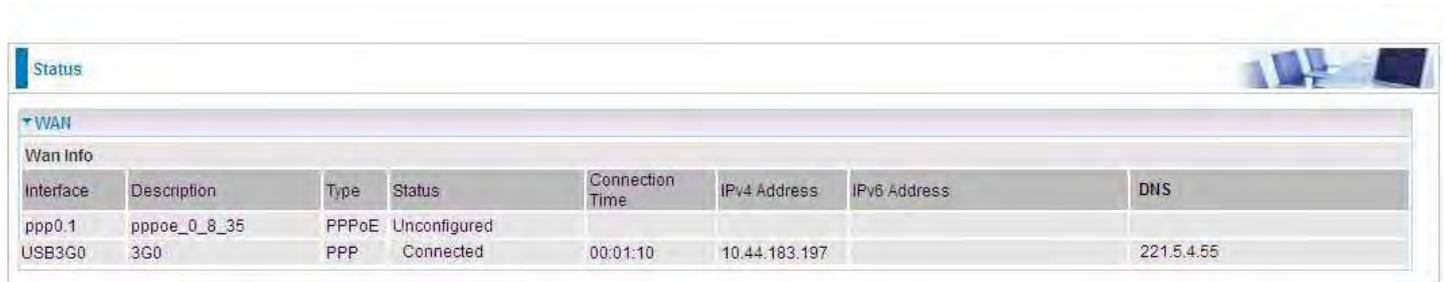
The screenshot shows a web interface with a 'Status' tab selected. Underneath, there is a 'WAN' section with a 'Wan Info' table. The table has columns for Interface, Description, Type, Status, Connection Time, IPv4 Address, IPv6 Address, and DNS. Two rows are visible: one for 'ppp0.1' (PPPoE, Unconfigured) and one for 'USB3G0' (PPP, Connected).
