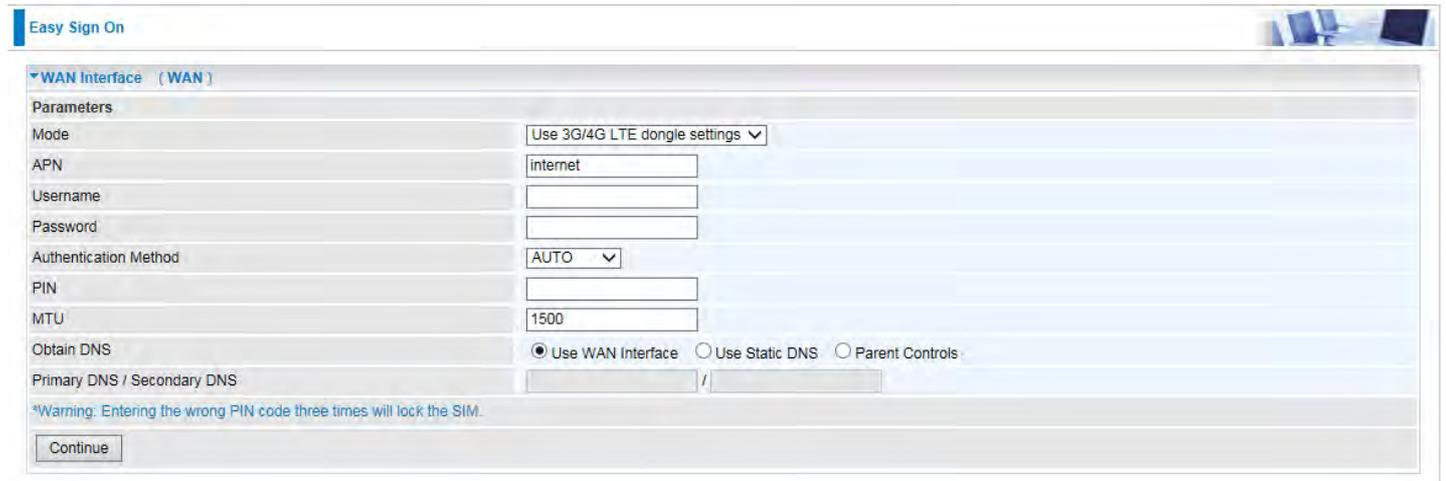
The screenshot shows the 'Easy Sign On' interface. The 'WAN Interface (WAN)' section is expanded to 'Parameters'. The 'Mode' is set to 'Use 3G/4G LTE dongle settings'. The 'APN' is 'internet'. The 'Authentication Method' is 'AUTO'. The 'MTU' is '1500'. The 'Obtain DNS' section has three radio buttons: 'Use WAN Interface' (selected), 'Use Static DNS', and 'Parent Controls'. There is a warning message: '\*Warning: Entering the wrong PIN code three times will lock the SIM.' and a 'Continue' button.
